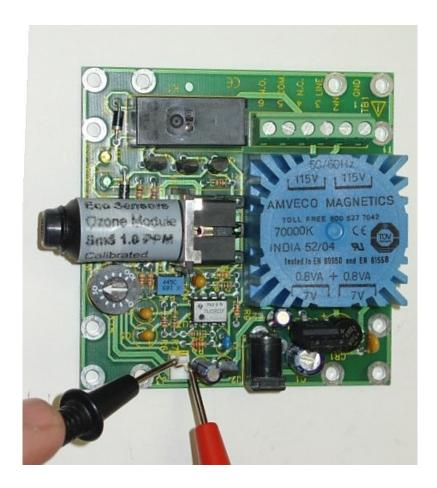
The voltage should read 1.0 volts when the sensor is exposed to ozone at the concentration of its full range.
