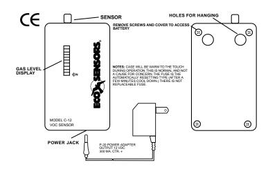
AC Adapter For use in North America and other areas with the "American System" of 120 V 60 HZ, the Eco Sensors P-20 adapter should be used. For other areas adapters should be purchased locally that fit local wall sockets and conform to local codes. The output should be 12 volts DC unregulated, 300-500 mA. The plug to our instrument should fit a 5.5/2.5 mm socket with the center pin +. For further details see our Tech Note P-101.
