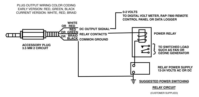
The C-21 internal relay is a "dry contact" FET device. It will handle up to 30 volts AC or DC at up to 130 ma so it will switch low voltage alarms directly. For switching power loads an intermediate relay and power supply should be used such as shown above.
