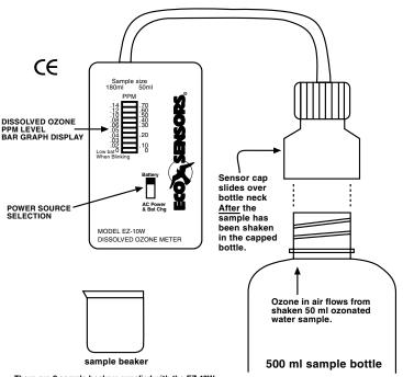
re are 2 sample beakers supplied with the EZ-10W: 50 ml for 0 -.7 ppm and 250 ml for 0 - .14 ppm
