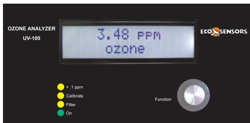
The Eco Sensors model UV-100 ozone analyzer is for general purpose measurement of ozone in air. Its range is .002-100 ppm (v) with 2% accuracy, and it includes a built-in data logger. The UV-100 weighs only 2.1 kg (4.7 lb), it is powered by an AC adapter or 12 V external battery, and is equally versatile for the laboratory or for process monitoring. The outputs are digital display, 0-2.5 VDC and 4-20 mA. The instrument features a low cost sample line filter with a Change Filter LED.
