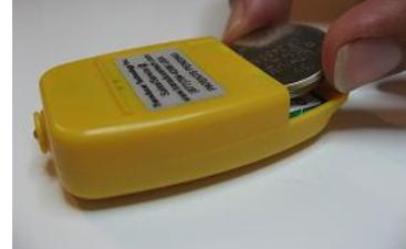
**3. Remove old battery. Wait 1 minute before inserting new one. \*Failure to follow procedure may cause the loss of calibration and void the warranty. *Check inside of battery cover for calibration due date.***
